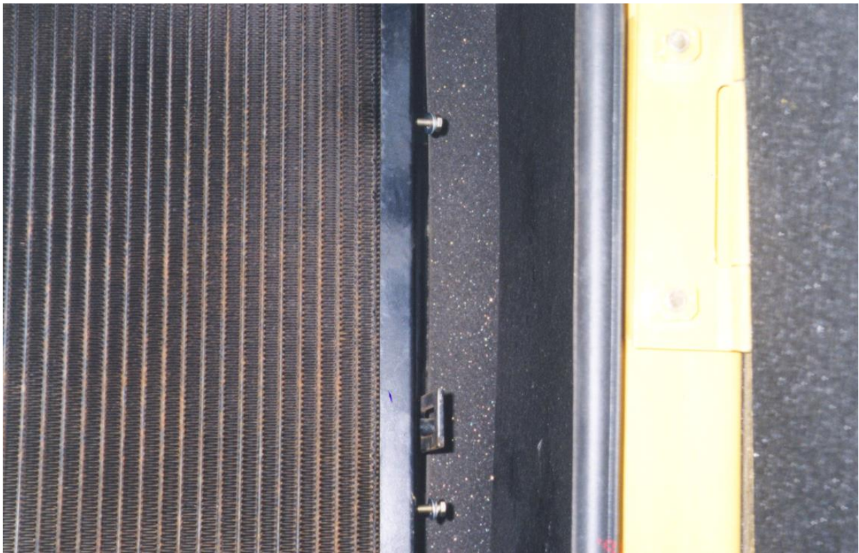
Condenser mounting positions indicated with hardware.
